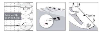
Measure the room to create a balanced layout. By measuring, you will be able to determine if the first row needs to be cut. The first and last rows should not be less than 5 cm wide.
