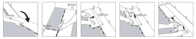
Always ensure that the short end joints are staggered by a minimum of 30 cm (= 3 click elements) when you start the next row. Use the leftover piece from the previous row as the first piece of the next row, provided that this piece is at least 30 cm long. In order to find a connection with the locking tabs of the previous row, it may be necessary to cut off an extra part of the leftover piece.
